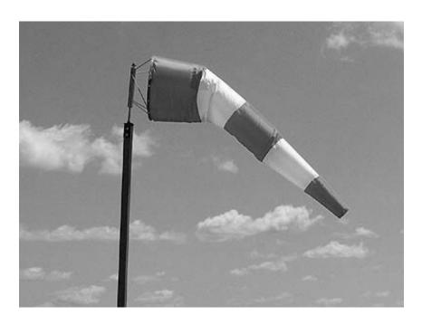
A windsock is a fabric tube designed to show the direction and speed of wind.
